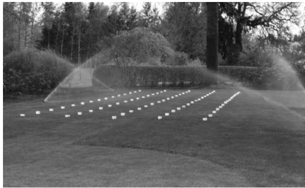
Figure 9-11 Can tests start with cans laid out on a grid. The system is run for a given amount of time, and the water collected in the containers is used to compute the precipitation rate, the distribution uniformity, and the scheduling coefficient. Adjustments are made as needed to improve coverage.
